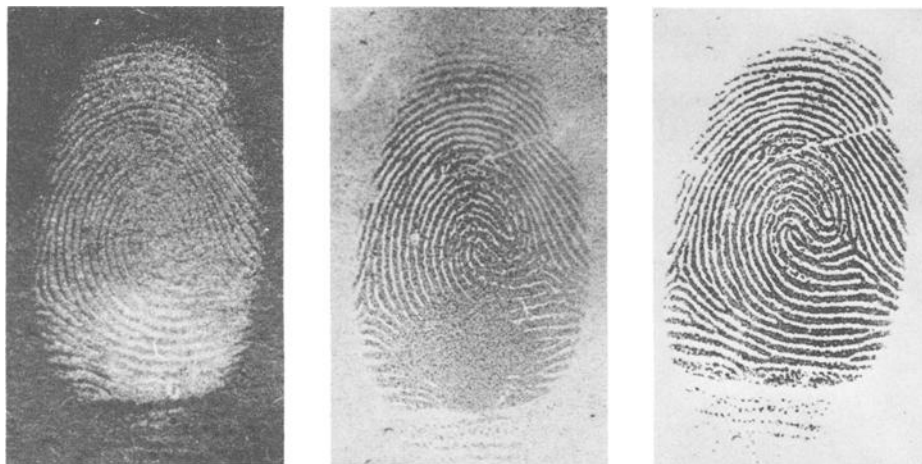
FIG. 1—Three different prints from the same finger: (left) print developed by anthranilic acid; (center) print developed by anthracene; and (right) inked print for comparison.
